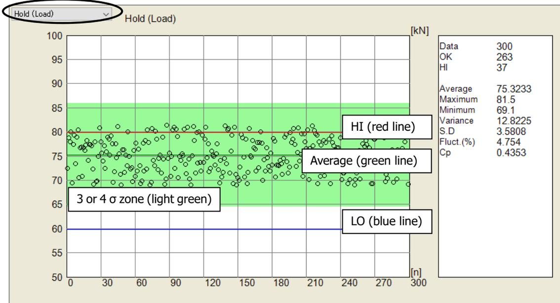
⇒ The horizontal axis is data number and the vertical axis is displacement or load.
