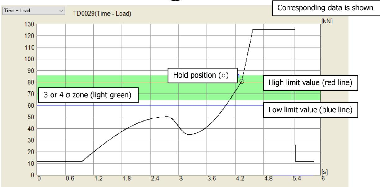
⇒ The horizontal axis is time and the vertical axis is displacement or load.
