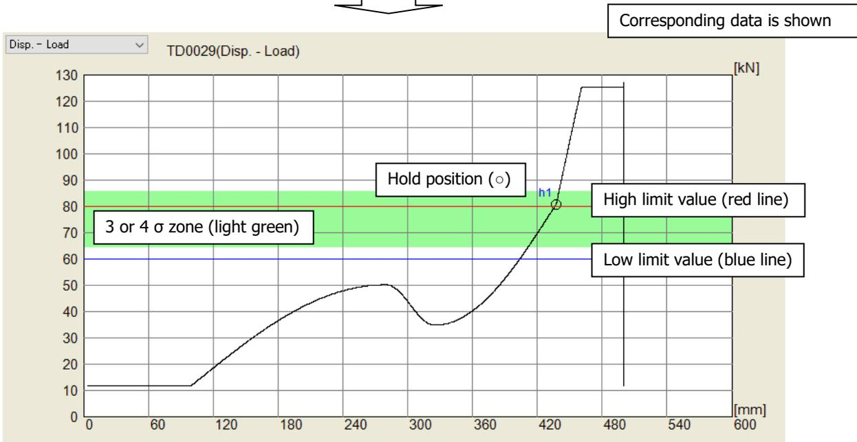
⇒ The horizontal axis is displacement and the vertical axis is load.
