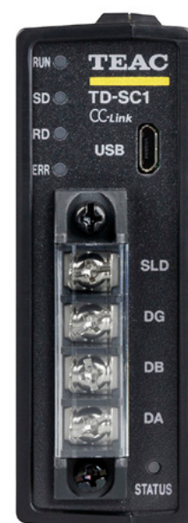
TD-SC1 (CCL) Industrial network CC-Link model
