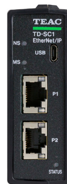
TD-SC1 (E/IP) Industrial network EtherNet/IP™ model
