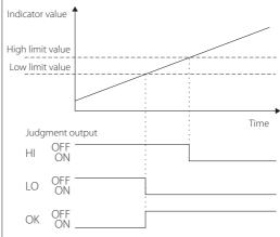
When set to LO/HI/OK, all are assigned to low limit (when Standard Comparison Output Pattern setting)
