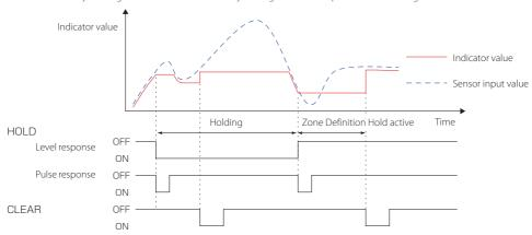
When holding, sending a Hold Clear command or making the control input terminal Clear signal ON will also reset the bottom value.
