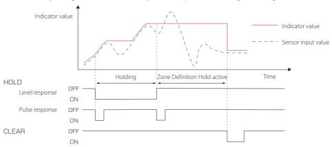
When holding, sending a Hold Clear command or making the control input terminal Clear signal ON will reset the peak value.
