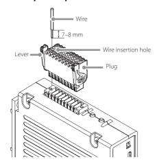
Remove 7 to 8 mm of the covering from the wire being connected, and twist it so that the tip does not come apart.
