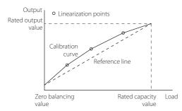
If linearization calibration is not conducted, a line connecting the two points between the zero balancing value and the rated capacity value will be used to calculate load.
