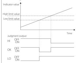
When set to OK/LO/HI, all are assigned to high limit (when Standard Comparison Output Pattern setting)
