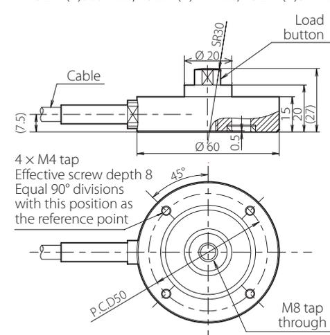
Dimensions in millimeters (mm)
