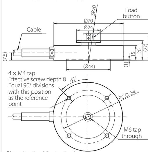
Dimensions in millimeters (mm)
