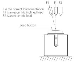
Refer to the following table for the allowable bending moment and allowable lateral load, and use it so that neither of these tolerances are exceeded.
