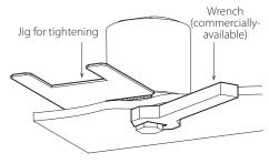
When tightening the screw or nut attached to the load cell, holding the screw/bolt part on the opposite end (shown with diagonal lines), will cause twisting force to be applied to the gauge and break the load cell.
