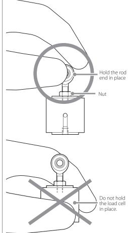
Always use screws/bolts that are suitable for the rated capacity when attaching a base plate or tensile load adapter, for example, to the load cell. Moreover, tighten all of the attachment screws/bolts evenly.
