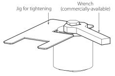
In the same way, when attaching a rod end or base, for example, to the screw/bolt area on the bottom of the load cell, use the included jig to hold the area shown with diagonal lines at the bottom and tighten the screw or nut.
